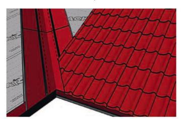
Install the cut panels up to the top of the valley, making sure as you proceed that the angle of the valley follows the guide line you have drawn.
