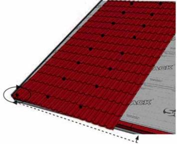
Remove the screw from ridge and align the panels with the eaves. This can be done by measuring to ensure that the length of the overhang is equal at the left and right corner of the sheet (approx. 1/4 - 1 inch).
