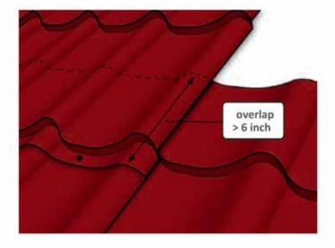
A panel is overlapped at the profile's stamp by at least 6 in. and fixed at the bottom of the wave into the decking below the stamp.
